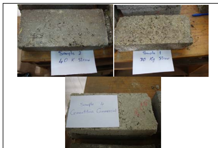
Figure-1. Rice straw cementitious and commercial cement brick samples under testing.
