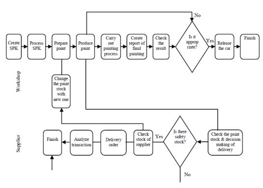
Figure-3. Process flow of To-Be scenario #2.
