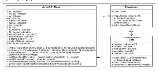
Figure-2. Class diagram for java BA implementation.
