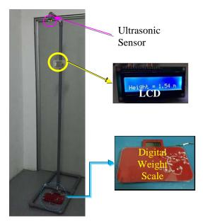
Figure-2. Prototype of measurement unit.
