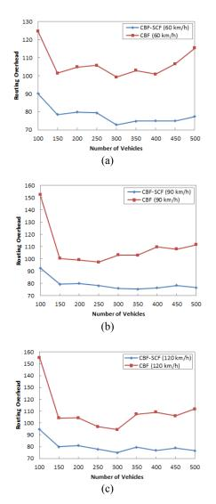
**Figure-8.** Routing overhead with different node speeds. (a) 60 km/h. (b) 90 km/h. (c) 120 km/h.
