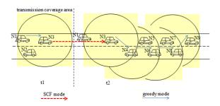
Figure-3. An illustrative example of CBF-SCF operation with respect to neighbors of the vehicleN3at different times t1 and t2.
