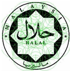
Figure-11. Detection of interest points in a Grayscale image using SURF.
