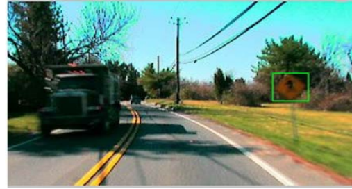
Figure-4. An example of frame with a detected sign from the video (Shneier, 2005).
