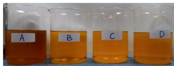
Figure-5. Colour of the oil samples, indicating the effectiveness of the reclamation process: (A) oil before reclamation, (B) oil after 5th reclamation cycle with Fuller's earth, (C) oil after 5th reclamation cycle with bentonite, and (D) oil after 5th reclamation cycle with PSAC.
