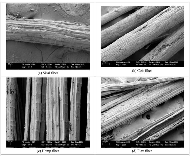
Figure-1. Scanning Electron Micrographs of NaOH treated fiber surfaces.
