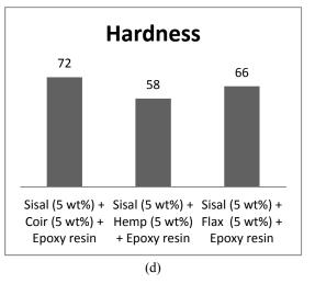
Figure-2. Mechanical properties of hybrid composites (a) Tensile, (b) Flexural, (c) Compression and (d) Hardness.
