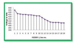
Figure-4 (a).Output voltage of existing system2 (Feeder1).
