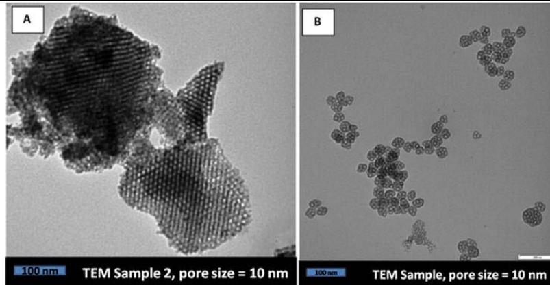
**Figure-5.** TEM images of MS-pure samples.**Table-1.** Cellulase loading capacity of non-functionalized (MS-pure and NS-pure) with open and blocked pores.
