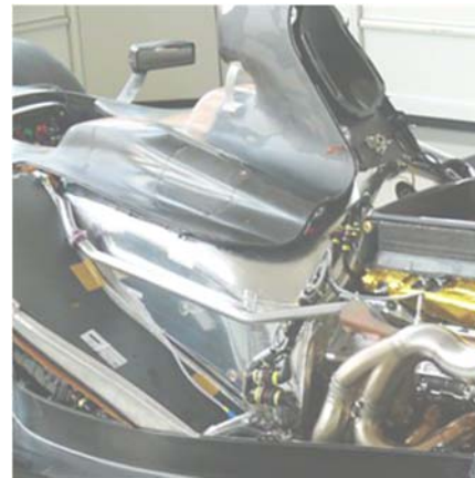
Figure-14. F1 radiator inclined along the pitch axis.
