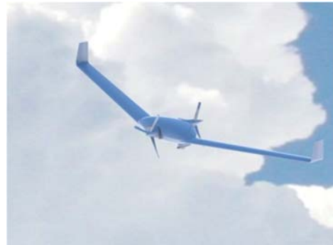
Figure-2. High altitude (20, 000m) UAV preliminary design with two contra-rotating propulsion units.
