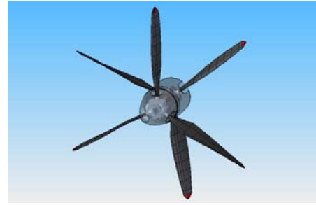
Figure-1. Propeller for 190kW/1250rpm/20km/0.4 M/ 2.5m diameter.
