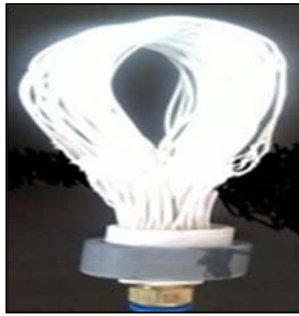
Figure-1. U-shape ultrafiltration membrane module.
