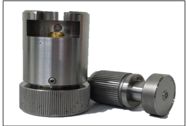
Figure-1. The high temperature probe with the calibration shorting block.
