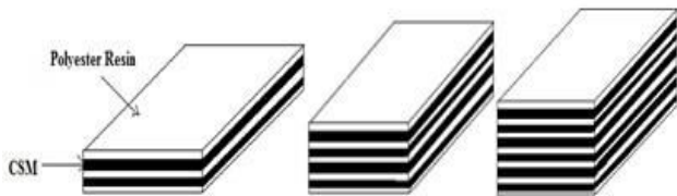
Figure-1. Two, four and six layers laminated CGRP composite.
