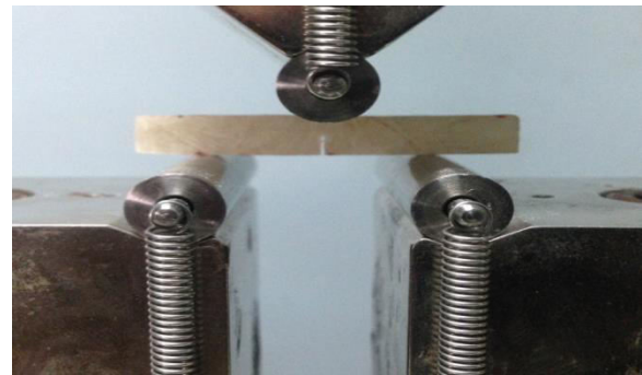
Figure-10. Fracture toughness testing in UTM.
