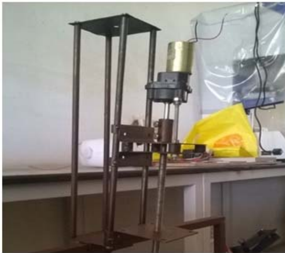
Figure-3. Dip coating machine.
