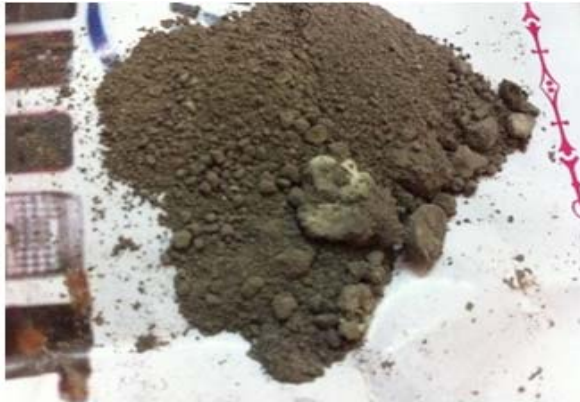
Figure-2. CeAlMn(x) powder using combustion synthesis.
