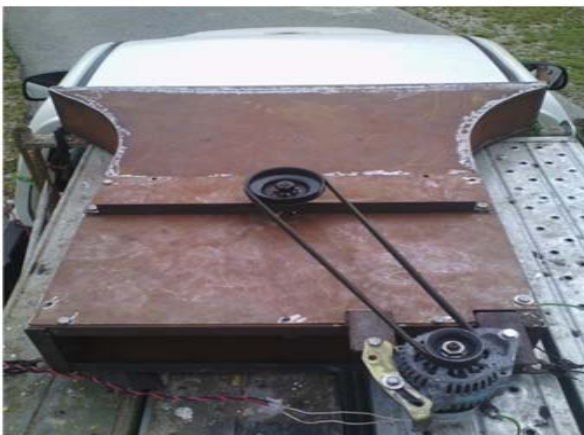
Figure-7. Installation of wind turbine on roof of pickup truck.
