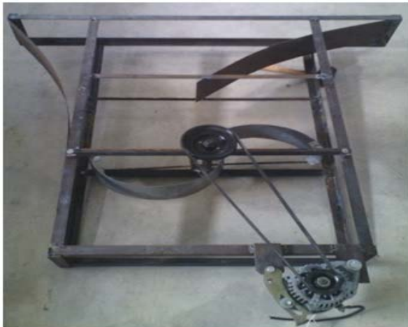
Figure-6. Installation of a wind turbine alternator.
