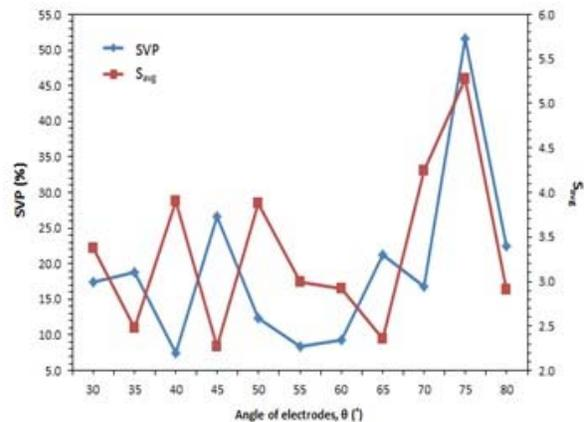
**Figure-4.** Effect of angles of electrodes on sensor sensitivity for four-plate sensors.
