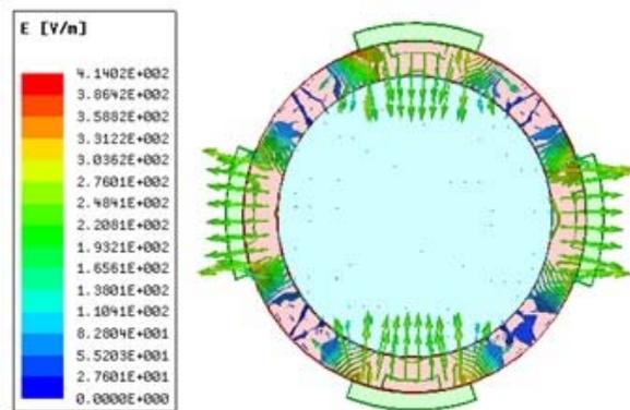
Figure-6. Electric field distribution of four-plate sensors.
