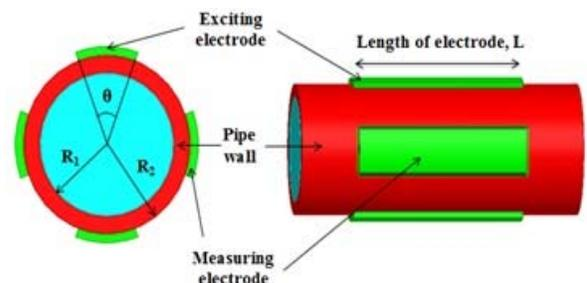
Figure-2. Electrode configuration of four-plate sensor.
