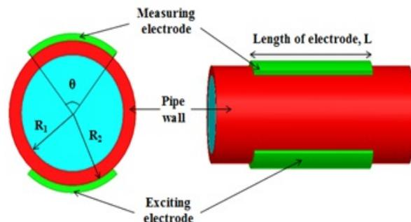
Figure-1. Electrode configuration of two-plate sensor.
