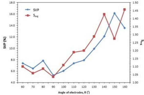
**Figure-3.** Effect of angles of electrodes on sensor sensitivity for two-plate sensors.
