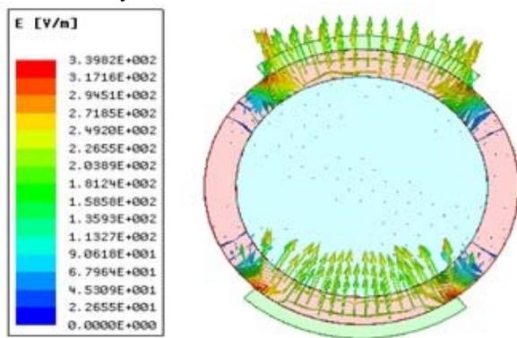
Figure-5. Electric field distribution of two-plate sensors.
