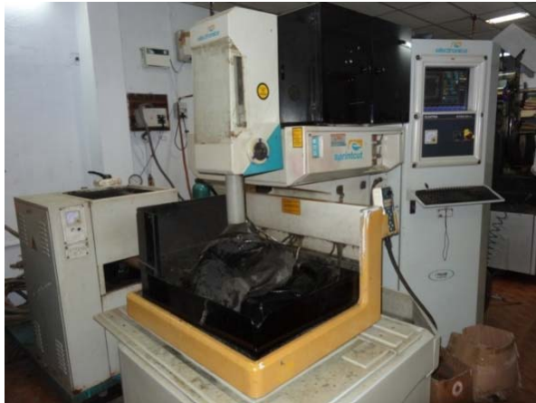
Figure-2. WEDM experimental set up (Electronica sprint cut).
