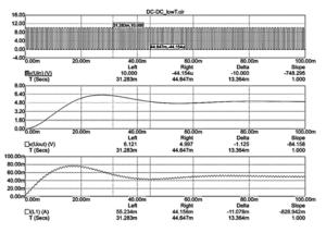
Figure-21. Voltage and current waveforms of a down DC-DC-converter with transistor switches.
