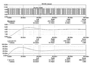
**Figure-19.** Voltage and current waveforms in the circuit of a down DC-DC-converter with a diode switch.
