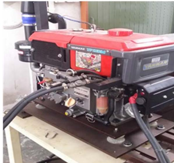
**Figure-2.** Yanmar diesel engine TF12ML.
