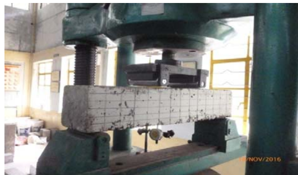
Figure-3. Flexure test on beam.
