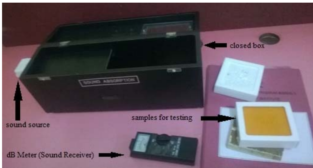
Figure-5. Photograph of the test set up.
