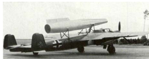
Figure-2. This Do 17Z with a 1.5m ramjet encountered serious stability and handling problems (1943) [7].
