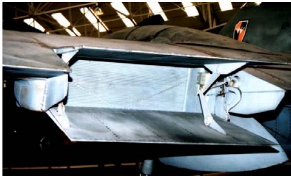
Figure-9. Bf109 with the nozzle fully opened (possibly a late G or K due to the absence of the boundary layer bypass duct).
