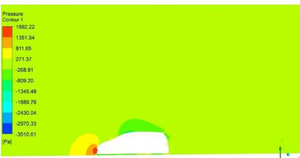
Figure-10. Pressure contour on symmetry plane.
