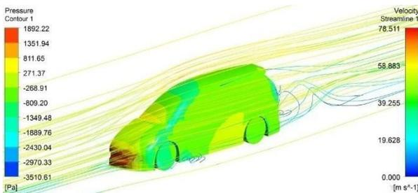
Figure-9. Pressure contour and velocity streamline
