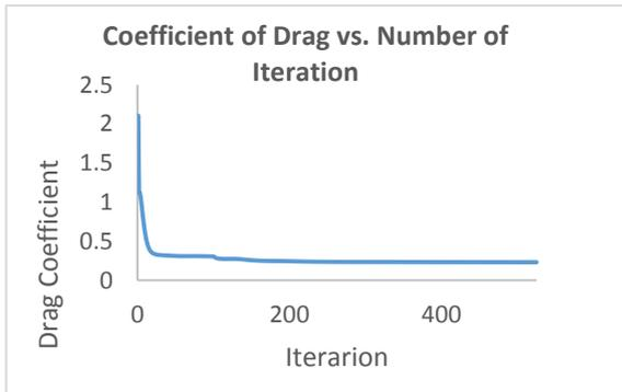
Figure-5.  $C_d$  vs. number of iteration.
