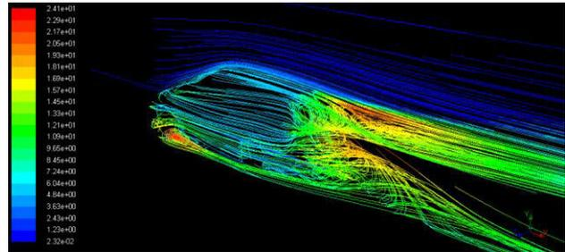
Figure-11. Turbulence intensities streamline (back).
