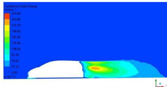
Figure-12. Contour of turbulence kinetic energy on symmetry plane.
