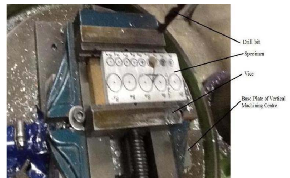
Figure-2. Drilling of prepared specimen in vertical machining centre.
