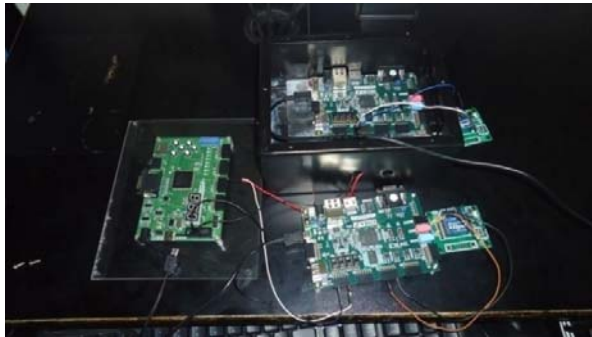
Figure-10. Hardware verification setup using client server nodes along with Spartan3 module.
