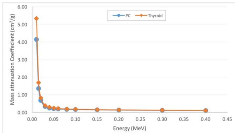
**Figure-2.** The mass attenuation coefficient of PC material compared with the human thyroid
