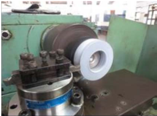
Figure-1. Experimental set-up of elastomer turning process.
