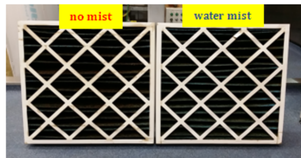
Figure-4. Pre-filter after reached maximum final resistance (pressure drop).
