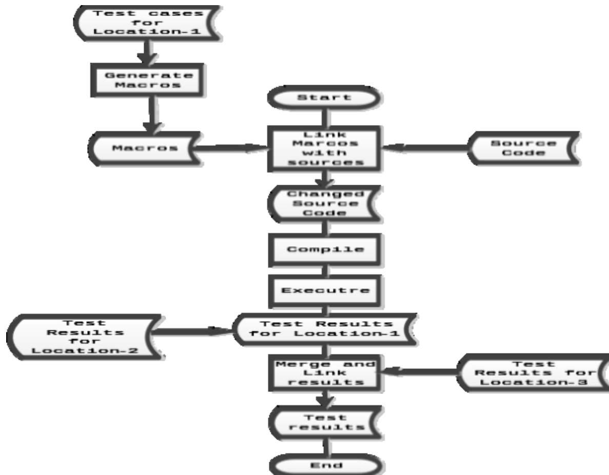
Figure-1. Process flow for undertaking testing using Assert Macros.
