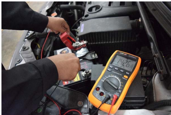
Figure-2. Measuring battery reading.
