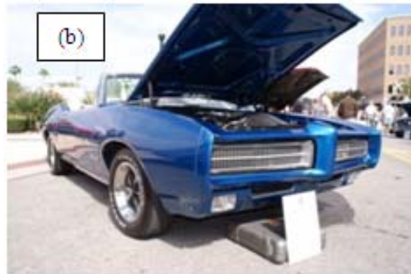
Figure-1. Car bumper; (a) Chrome plated front bumper made from metal assembled at Ford Taunus in 1958 and (b) front bumper made from plastic assembled at Pontiac GTO in 1968 [2].
