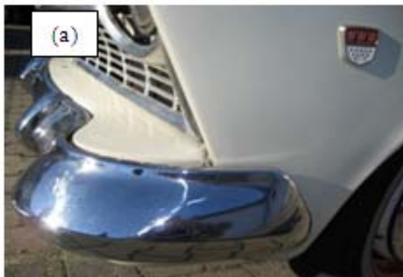
Figure-1. Car bumper; (a) Chrome plated front bumper made from metal assembled at Ford Taunus in 1958 and (b) front bumper made from plastic assembled at Pontiac GTO in 1968 [2].
