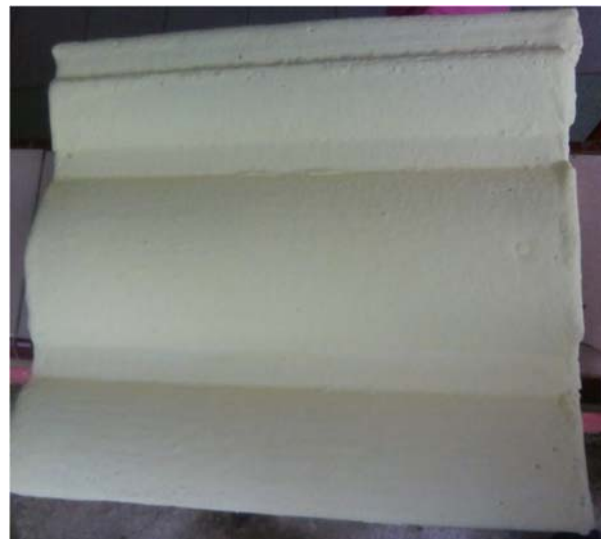
Figure-13. Application of lightweight concrete and coating used as roof tiles.
