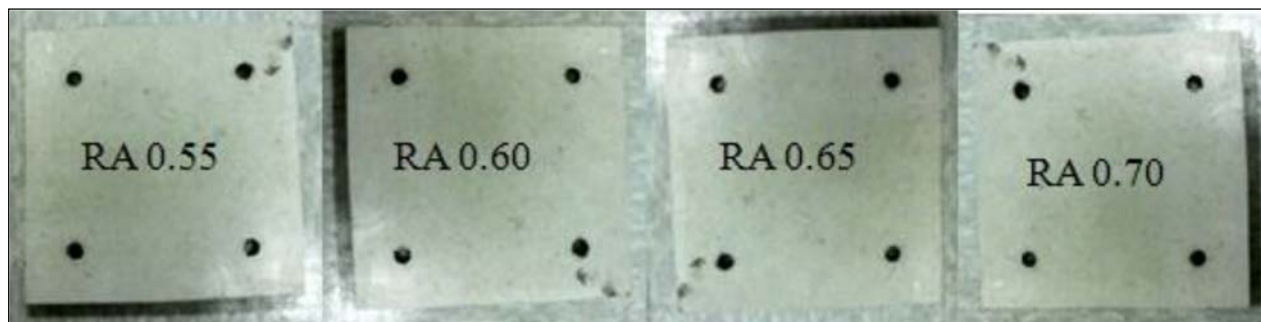
Figure-1. Sample for vibration test with different portion of rubber aggregate; 0.55, 0.60, 0.65 and 0.70 weight to weight (wt/wt).
