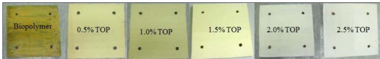
Figure-2. Specimen for vibration test for coated lightweight concrete with different percentages of biopolymer doped with titanium dioxide (0.5, 1.0, 1.5, 2.0 and 2.5 %).
