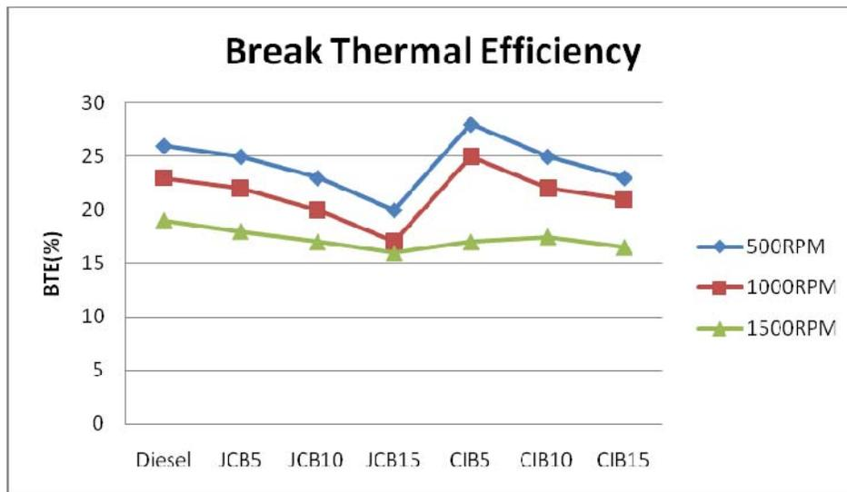
**Figure-3.** Brake thermal efficiency at multiple idling situations for diesel, Jatropha curcas biodiesel and Calophyllum.
