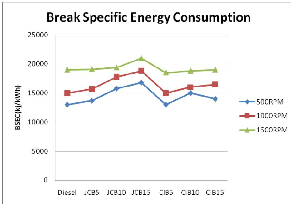
**Figure-2.** Brake specific energy consumption at multiple idling situations for diesel, Jatropha curcas biodiesel and Calophyllum biodiesel blend.
