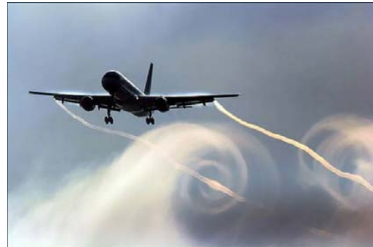
Figure-2. Boeing 767 showing wing-tip vortex.
