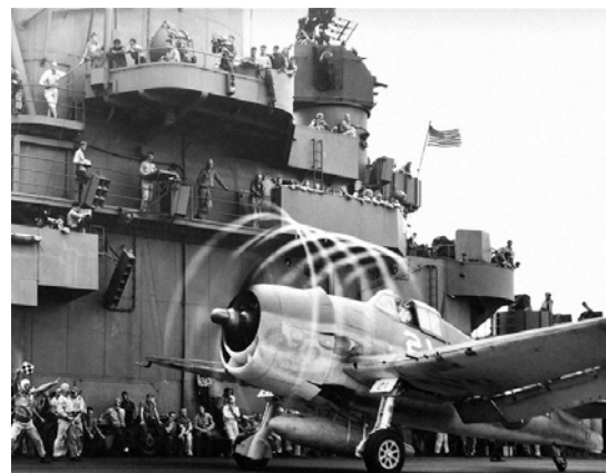
Figure-3. propeller tip vortices of a Grumman F6F Hellcat.
