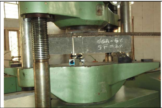
Figure-4. Flexural strength set-up.
