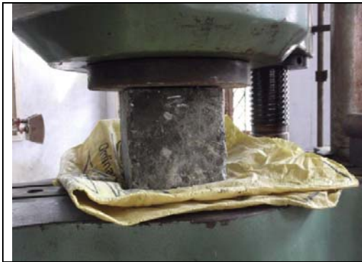
Figure-3. Compressive test set-up.
