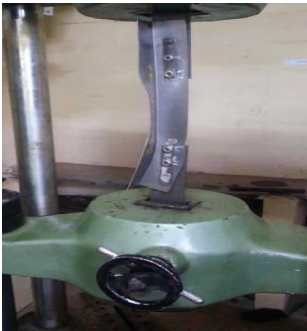
Figure-6.a. Single plain angle without lip (2mm).
