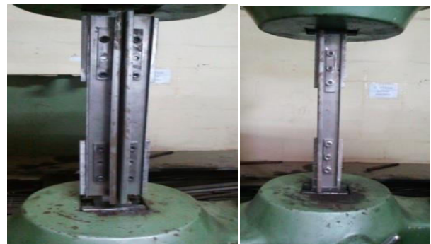
Figure-4. Angles fixed in universal testing machine (UTM).
