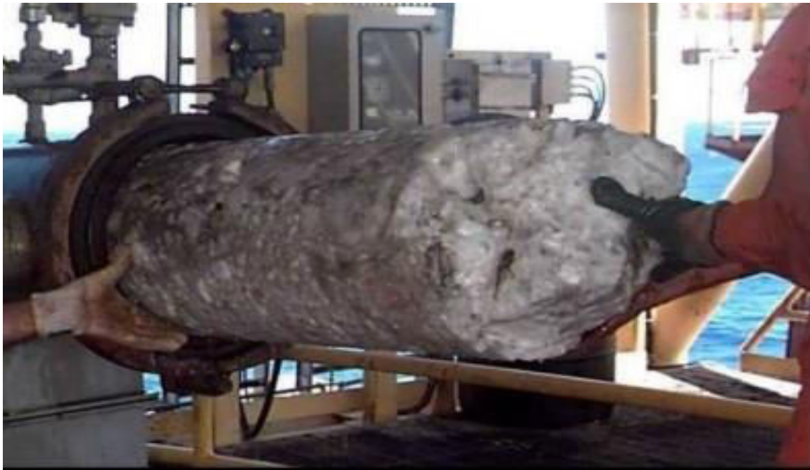
Figure-1. A large gas hydrate plug formed in a subsea hydrocarbon pipeline. Source: Heriot-Watt University Institute of Petroleum Engineering, (2013).
