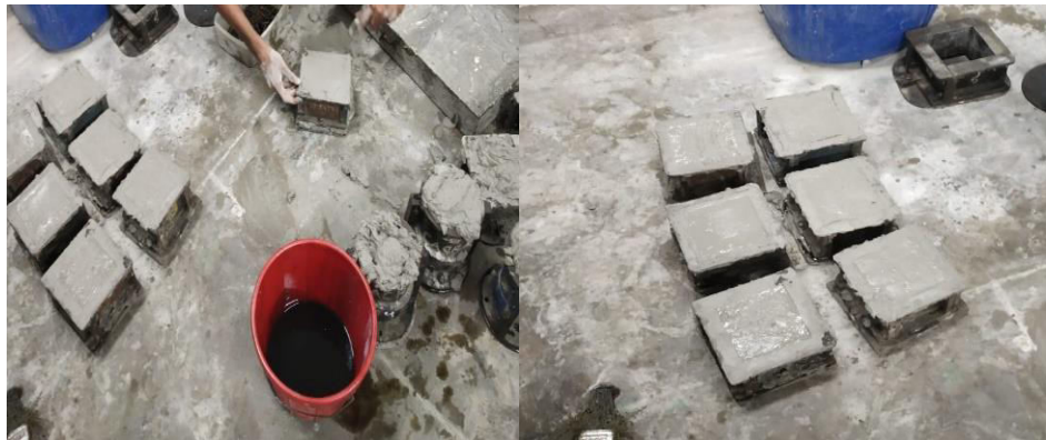
Figure-2. (a) & (b) Casting of specimens.
