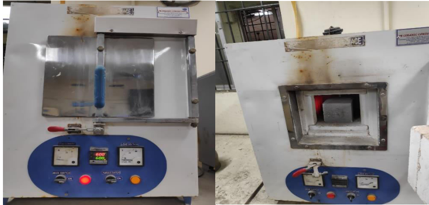
Figure-5. (a) Electric furnace (b) Specimen inside the electric furnace.
