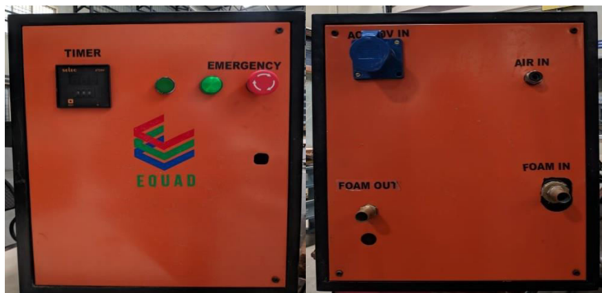
Figure-1. (a) Front side of foam generator (b) Back side of the foam generator.
