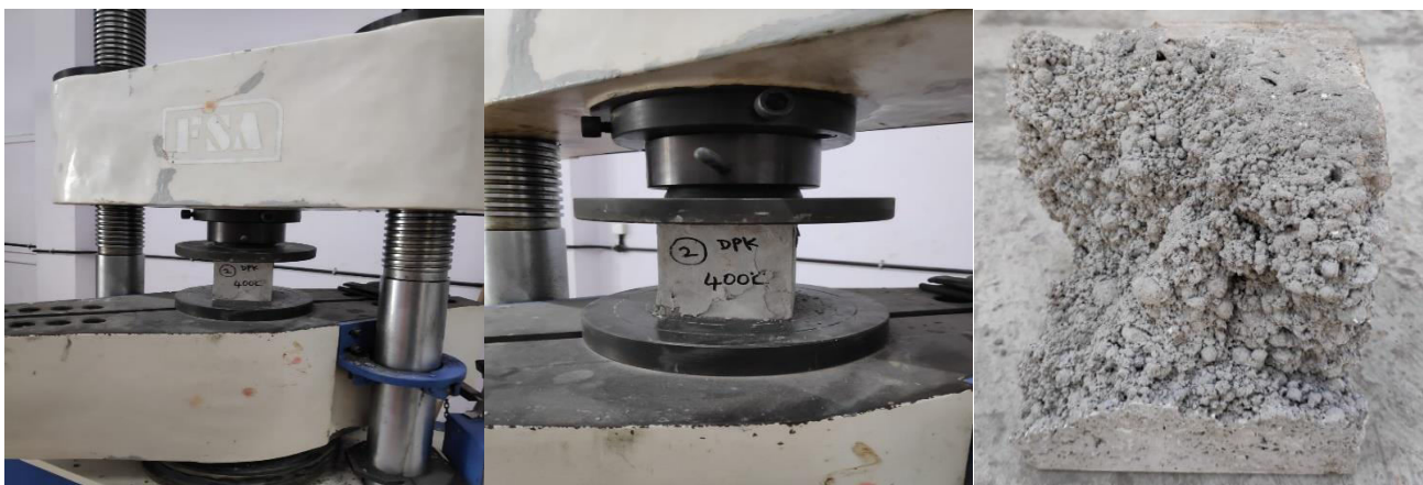
Figure-4. Compressive strength test (a) compressive strength test in CTM (b) failed specimen (c) Air bubbles inside the failed specimen.
