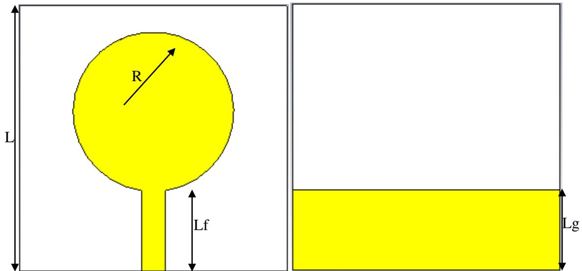
**Figure-1.** Basic circular patch antenna with DGS.
