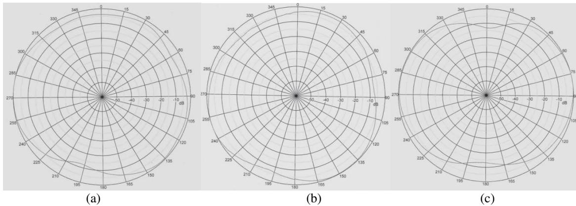
**Figure-10.** (a)-(c) Measured radiation patterns of proposed antenna at 5.0 GHz, 8.0 GHz, 12.0 GHz respectively.
