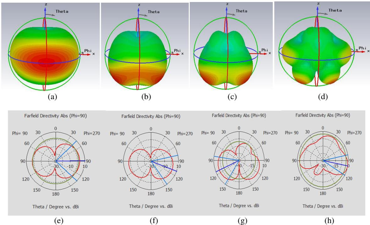
Figure-3. (a)-(d) 3D Radiation patterns (e)-(h) 2D Radiation patterns at 4.1 GHz, 6.7 GHz, 7.5 GHz and 12.6 GHz frequency.
