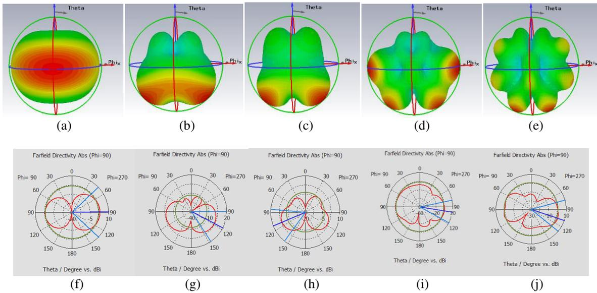
**Figure-9.** (a)-(e) 3D radiation patterns (f)-(j) 2D radiation patterns of proposed antenna at 4.1 GHz, 7.5 GHz, 8.5 GHz, 12.5 GHz and 15.4 GHz respectively.
