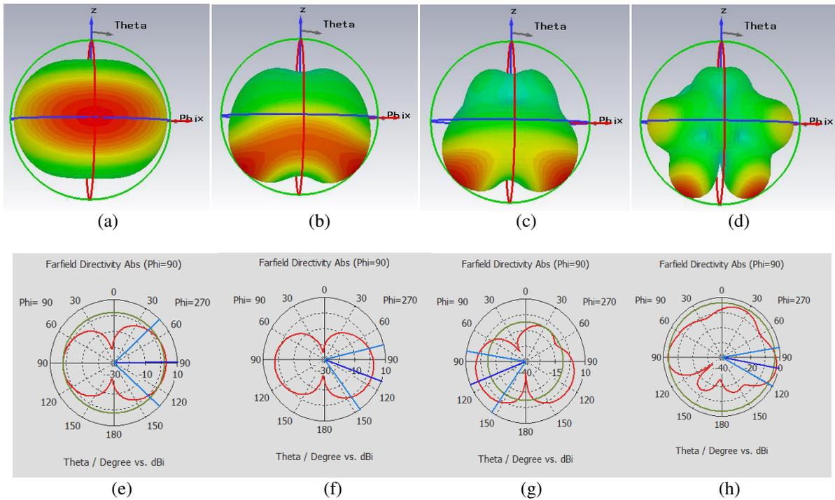
**Figure-6.** (a)-(d) 3D Radiation patterns (e)-(h) 2D Radiation patterns at 4.1 GHz, 6.7 GHz, 7.5 GHz and 12.6 GHz frequency.
