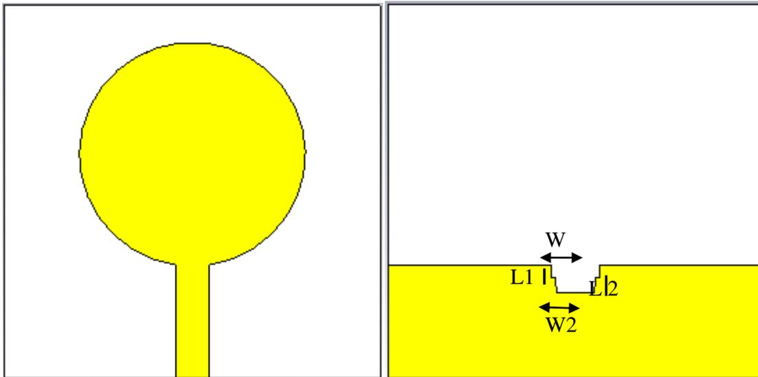
**Figure-4.** Circular patch antenna with modified DGS.
