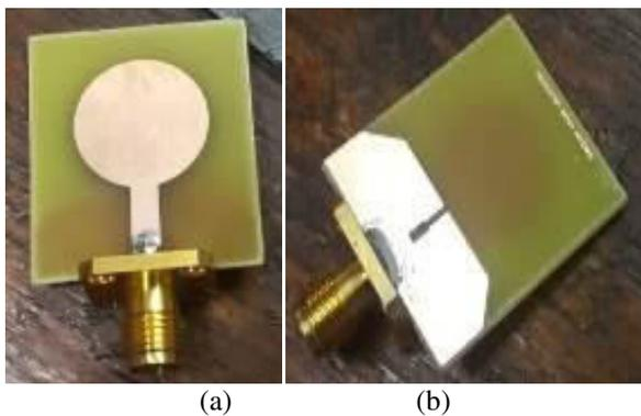
**Figure-11.** Fabricated Prototype of proposed antenna (a) Front view (b) back view.
