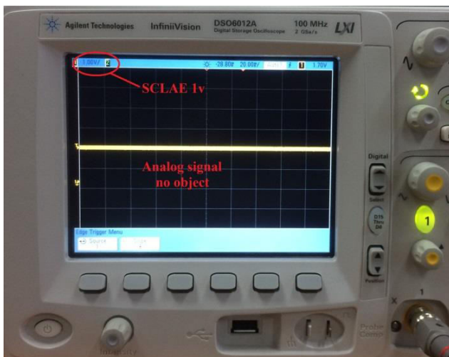
Figure-14. Oscilloscope display in the absence of an object with an analogue output.
