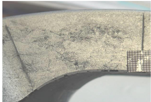
Figure-4. Cluster of oxide spots on the outer surface of cast.
