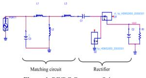
Figure-1. RF/DC Converter Schema.
