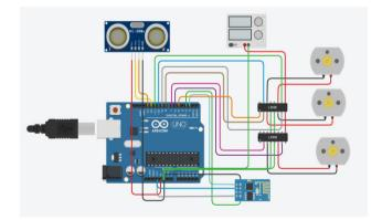
Figure-2. Connection of Multi-Controlled Floor Vacum Cleaner.
