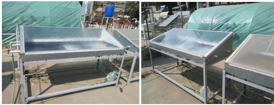
Figure-1. L-type solar stiller during desalination of seawater and recovery of fresh water at the bottom.
