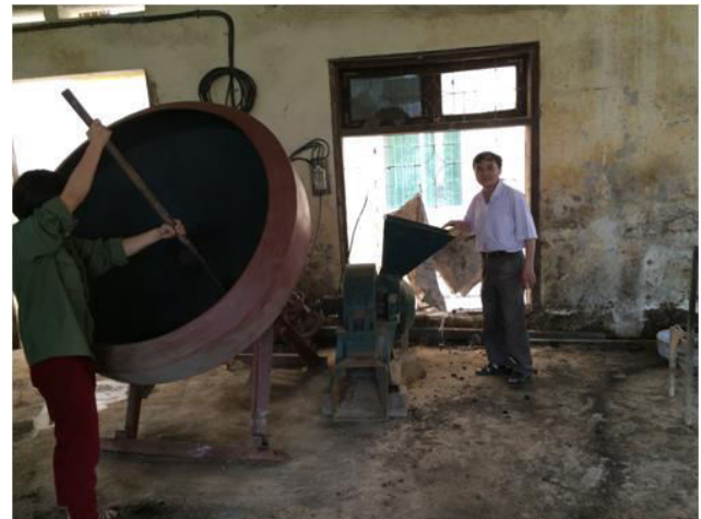
Figure-1. Mixer Machine and Pellet Machine in NPK-Biochar fertilizer production.
