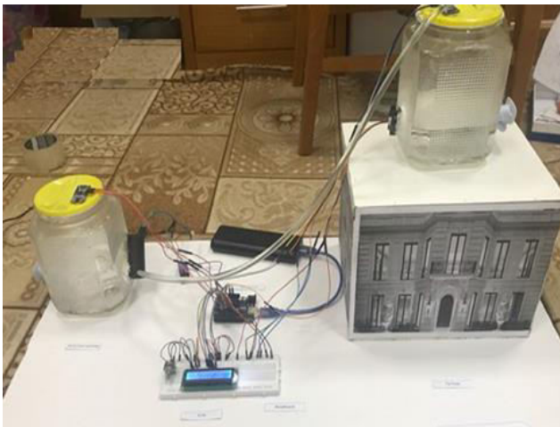
Figure-5. Side view of prototype of the proposed automated system for water tank monitoring.
