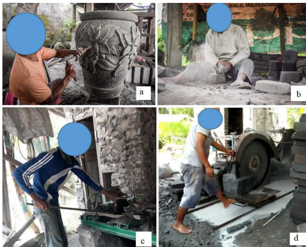
Figure-1. Activities on traditional stone carving industry: (a) carving, (b) grinding, (c) turning, and (d) sawing.
