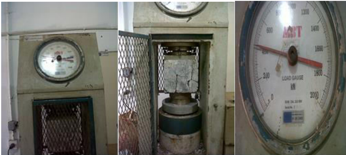
Figure-5. Display of testing of concrete compressive strength for selected concrete quality.
