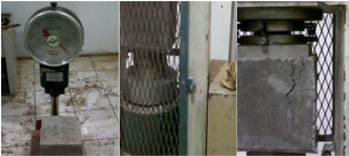
Figure-4. Display of dial for normal concrete compressive strength.
