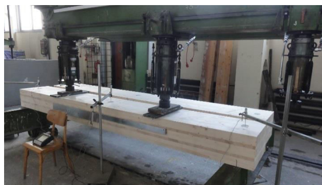
Figure-1. Tested specimen subjected to a four-point bending test.
