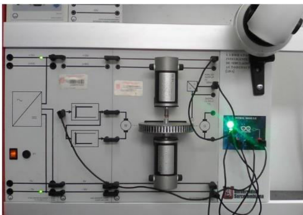
Figure-14. Final hardware product for remote LISA.
